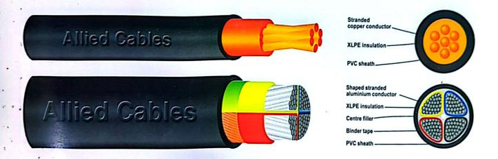
Single core and multicore cables with copper or aluminium XLPE insulated, armoured overall PVC sheathed 600/1000 V and 1900/3300 V conforming to IEC-60502
